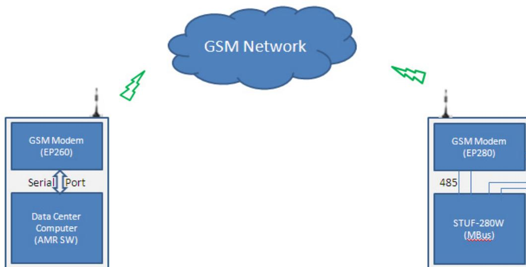
Figure 5. AMR system reads GSM-enabled water meter directly.
