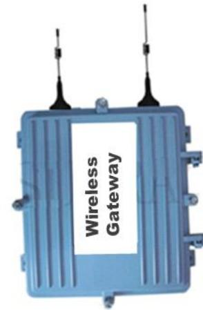
The Wireless Gateway has two wireless modems, one is GPRS modem which communicates with data center through GPRS cellular network, the other is RF wireless modem which communicates with WDLR through 470MHz radio wireless. It has a voltage stabilized switching power supply, which ensures its reliable operation in complicate power supply environment.
